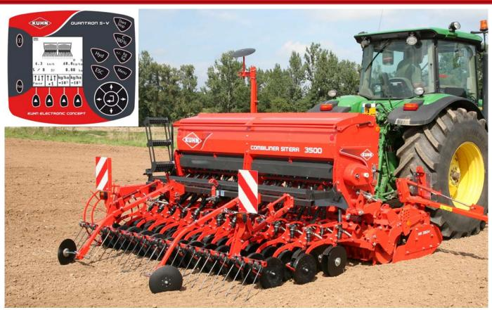
To benefit from electronic seeding application rate adjustment during operations, the PREMIA and SITERA mechanical seed drills can now be equipped with a QUANTRON S control box. Adjustment is achieved via an electric cylinder acting directly on the selector control lever.
